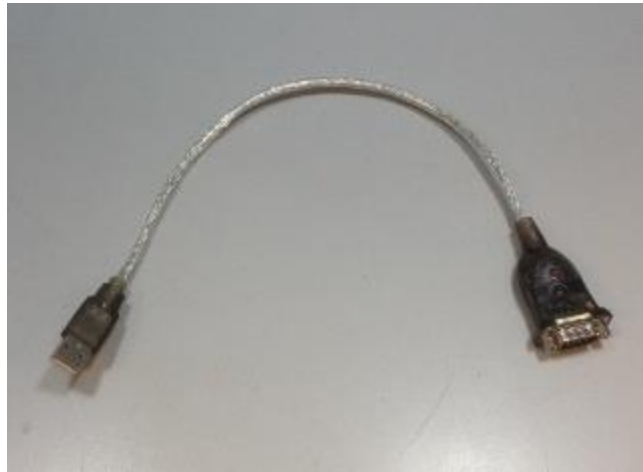
Figure 164. RS-232 to USB Converter for Connection via USB Port
