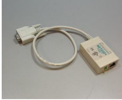
Figure 163. Ethernet to RS-232 Converter for Connection via Serial Port
