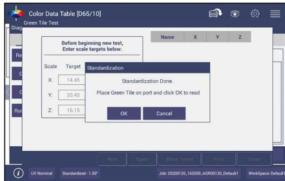
Figure 66. Input Target Values for Green Tile
