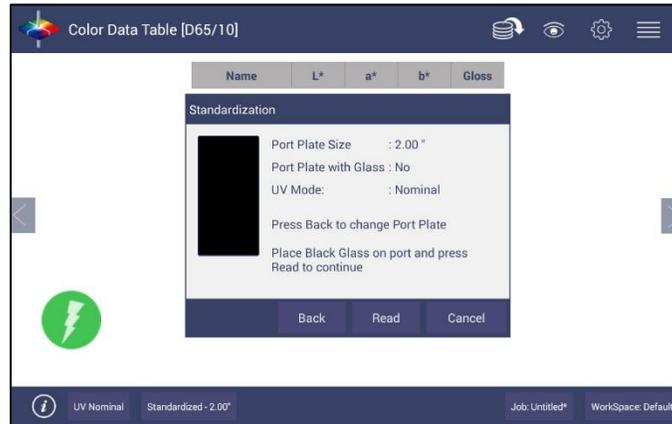
Figure 6. Read the Black Glass for Bottom-of-Scale
