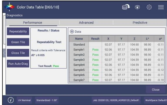
Figure 65. Diagnostics Repeatability Test Results
