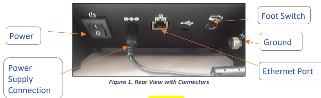
Figure 1. Rear View with Connectors
