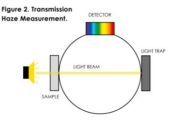
In order to compare results obtained for these various geometries, four samples were measured for haze on a sensor as prescribed in ASTM D1003 and then measured on different HunterLab d/8° sphere instruments. The values obtained are shown in the table below.
