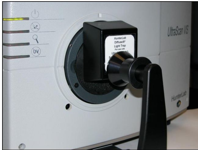
Figure 21. Standardizing with the Light Trap
